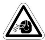
Airborne particles and loud noise hazards. Wear eye and ear protection.
