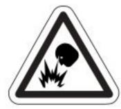
Take action to prevent static sparking. Fire or explosion can result, especially when handling flammable liquids. The pump, piping, valves, containers and other miscellaneous equipment must be properly grounded.
