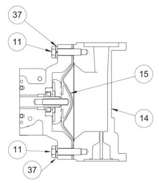
Diaphragm Orientation Install diaphragm and spacer
