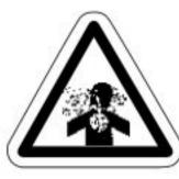
In the event of diaphragm rupture, pumped material may enter the air end of the pump, and be discharged into the atmosphere. If pumping a product that is hazardous or toxic, the air exhaust must be piped to an appropriate area for safe containment.
