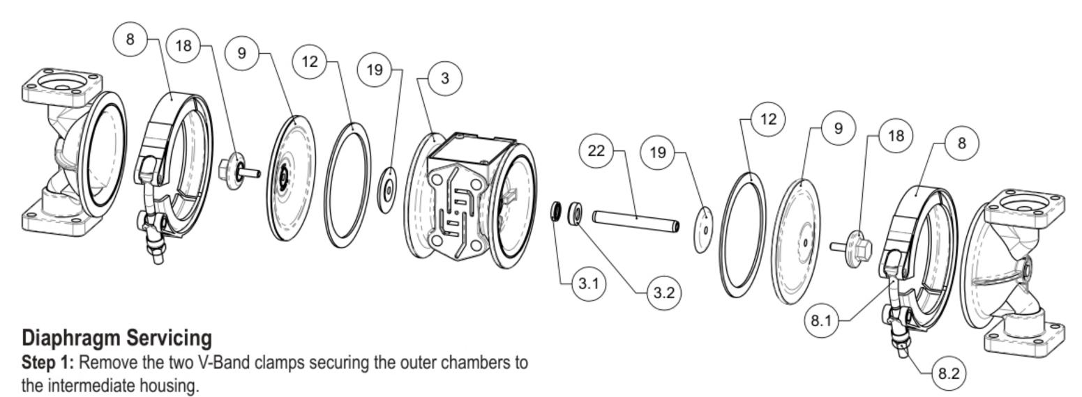
Step 2: Remove the diaphragm assembly (outer plate, diaphragm, spacer gasket (for PFTE units only, inner plate) by turning the assembly counterclockwise using a 1/2" (1.27 cm) wrench on the outer plate lugs. (If a socket is used, it must be a six-point socket.) The interior components
