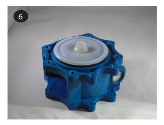
The other diaphragm(s) (item 17) and inner/ outer plates (items 19 & 23) can be installed onto the opposite end of the shaft (item 27). It may be easier to thread the molded in bolt into the shaft if the diaphragm(s) is inverted on one or both sides. This can be done by hand. 8 Tighten and torque the outer plates (item 19) to 40 in-lbs (4.5 N-m).
