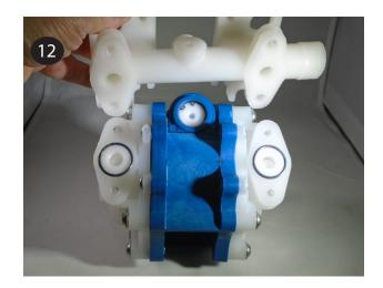
B Stand the pump upright onto the suction manifold feet (item 12). Place the valve balls (item 15), valve seats (item 14), and seat o-rings (item 13) into the discharge manifold (item 16) in the same order as the suction side was done in step 11. Place the discharge manifold atop the pump, tighten, and torque the discharge manifold bolts (item 11) in an "X" pattern. Torque to 50 in-lbs (5.6 N-m).
