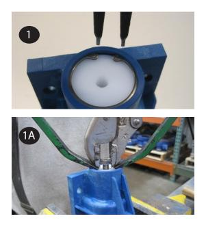
Plastic Air Valve - Remove and replace o-rings. Insert cap (item 6) push down until groove for the retaining ring is visible. Make sure to lubricate the o-rings prior to inserting into the valve body with a compatible lubricant.
