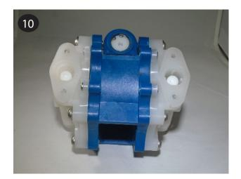
Place the valve seats (item 14) into the seat bore then the valve seat o-rings (item 13) into the groove that is formed by the seats. Place the suction manifold (item 12) atop the pump. Tighten and torque the suction manifold bolts (item 11) in an "X" pattern. Torque to 50 inlbs (5.6 N-m)
