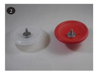
3 Apply a medium strength thread locker, such as Loctite<sup>®</sup> 246, to the outer plate (19) bolt threads and shaft (item 27) threads. To ensure thread locker cures quickly, a primer such as Loctite<sup>®</sup> SF7649 should be used. Thread the shaft onto the outer plate bolt until it is snug.
