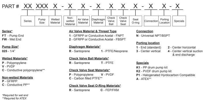
Example Pump P/Ns: FT025P-P1-RRPR-N1, FT025P-P1-1TPC-N1, FT025V-P1-1TVC-N1 & FT025C-C2-RRCR-N1-A Example Wet End P/Ns: FW025P-RRPR, FW025P-1TPC, FW025V-1TVC & FW025C-RRCR
