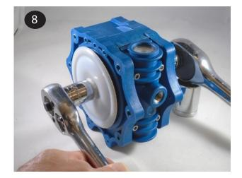
Install the liquid chambers (item 18) by placing one side over the diaphragm. Start all 6 screws (item 11) before tightening and torqueing. Torque all fasteners in a star pattern to 50 in-lbs (5.6 N-m). Start all 5 screws (item 17) before tightening and Torqueing. Torque all screws in a X Pattern to 30 in-lbs (3.4 N-m). Repeat to install the second liquid chamber. Ensure both chambers are orientated the same and that the inlet and outlet ports are vertical when facing the front of the pump.
