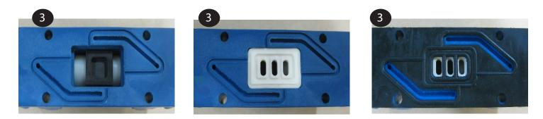
Insert the (4) cap screws (item 1) through the valve body and gasket (items 2 & 10) and place onto the center section (item 8). Ensure the slide valve and valve plate (items 8 & 9) are in place and the valve sits flat on the center section.
