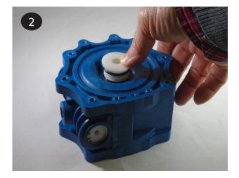
If replacing the bushings (item 24), then the muffler felt (NS) should also be replaced prior to replacing the second bushing. It is important when installing the felt that it does not block the air slot. Lubricate the bushing o-rings (item 25) and press it into the open bushing gland. Reinstall the bushing, hold down screw (item 17).
