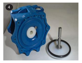
**5** For PTFE fitted pumps place the large diaphragm o-ring (item 21) into the groove in the center section (item 28).
