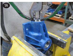
Plastic Air Valve - Remove and replace o-ring (item 5). Insert cap (item 6) and push down until groove for the retaining ring is visible. Install retaining ring. Make sure to lubricate the o-rings prior to inserting into the valve body with a compatible lubricant.
