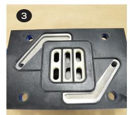
Insert the (4) cap screws & washers (items 1 & 2) through the valve body and gasket (items 3 & 36) and place onto the center section (item 35). Ensure the slide valve and valve plate (items 9 & 10) are in place and the valve sits flat on the center section.
