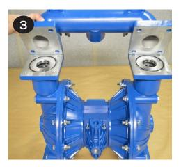
Remove both liquid chambers (item 18) by removing the (12) bolts & nuts (item 16, 17, & 27) on each liquid chamber using a 15 mm wrench. Inspect and replace diaphragms if needed.
