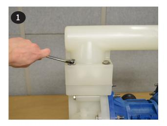
The discharge seat o-rings, valve seats, and valve balls (items 14, 15, 16, & 17) can now be accessed and replaced if needed.
