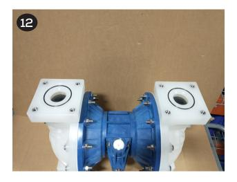
Place the manifold o-rings (item 15) into the o-ring gland on the suction manifold (item 13). Place the suction manifold atop the pump and install, tighten and torque the (8) manifold bolts & washers (items 11 & 12).
