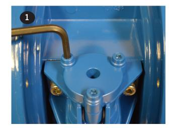
Plastic Air Valve - Remove and replace o-rings (item 5). Insert cap (item 6) and push down until groove for the retaining ring is visible. Install retaining ring (item 8). Make sure to lubricate the o-rings prior to inserting into the valve body with a compatible lubricant.
