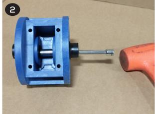
Use the supplied grease packets to lightly grease the OD and ID o-rings (items 28 & 30) that come preinstalled in the new shaft bushings supplied in air end kits.
