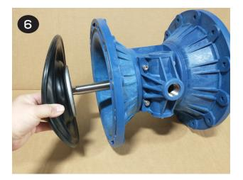
To remove the remaining diaphragm(s) (items 21/22) and plates (items 20 & 23) from the shaft (item 31), place the shaft in a vise. Using a 6-sided 30 mm wrench, remove the remaining diaphragm(s) and plates.
