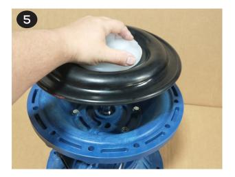
The may be easier to thread the molded in bolt into the shaft if the diaphragm(s) is inverted on one or both sides. This can be done by hand.
