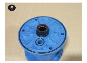
Install both air chambers (item 26) by placing one side on top of the center section (item 34). Ensure the air path hole of the center section lines up with the through hole in the air chamber. Insert the bolts & washers (items 24 & 25) through the air chamber and center section.
