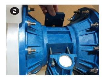
Place the new gasket (item 35) on the air valve (item 3) and ensure the slots in the gasket align with the slots in the air valve and valve plate (item 10).
