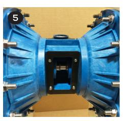
Tighten and torque the (4) cap screws into the muffler plate.
