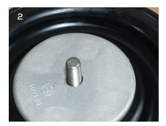
3 Apply a couple drops of a medium strength thread locker, such as Loctite® 246, to the molded in outer plate bolt (item 20). Thread the shaft (item 31) onto the molded in bolt until it is snug to the flat back side of the inner plate (item 22).
