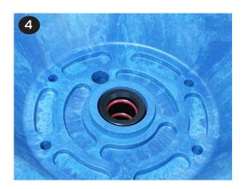
**5** Push the shaft (item 31) through the center of the shaft bushing (item 29). It is normal for this to be a tight fit, especially if the shaft and shaft o-rings (item 30) are in good condition.
