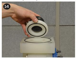
Place the valve balls (item 17) on the valve seats and discharge manifold (item 38) atop the components that are stacked on top of the liquid chambers. Install, tighten and torque the (8) manifold bots & washers (items 11 & 12).
