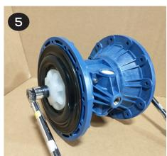
Remove the outer plate, diaphragm(s), and inner plate (items 20, 21/22 & 23) from the side that is loosened. Pull or push the shaft (item 31) and remaining plates and diaphragms out of the center section. If pulling, it may be easier to grip the diaphragm if it is inverted.
