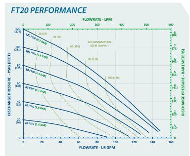
Full stroke diaphragm allows performance to be equal for all diaphragm materials
