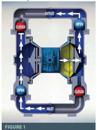
As the common shaft located in the center section moves to the right, the diaphragm in the left chamber moves towards the center section. This movement creates a vacuum on the liquid side of the left diaphragm, lifting the lower ball check valve, allowing liquid to flow through the suction manifold into the liquid chamber. At the same time, any fluid in the right chamber is discharged.
