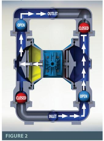
The air distribution system senses that the diaphragm in the right chamber reaches the end of its discharge stroke and causes the common shaft to shift. This moves the diaphragm to the left pressurizing the liquid, lifting the upper ball check valve, allowing fluid to flow though the discharge manifold and out of the pump.
